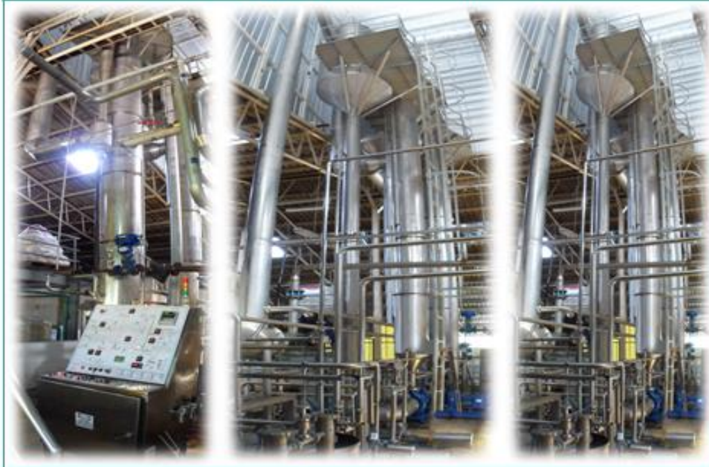
Double Effect Long Tube Force Circulation Evaporator For Coconut Milk, located at Ampol Food Processing Ltd., Thailand
